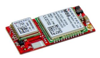
The KCS TraceME TM-231 / R9M2 is one of the smallest and lightest GPRS/GPS track-and-trace units of the world. It is targeted for tracking a variety of very small objects, or even small animals e.g. small birds.
